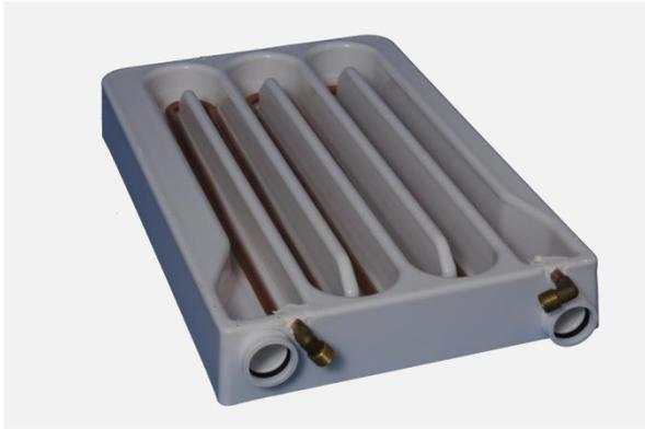
With an open lid it is easy to see how the heat exchanger works. The 3 m copper pipe efficiently transfers the heat. The greywater flows in the canal while heating the incoming coldwater inside the copper pipe. This design has increased efficiency due to the true counter flow heat transfer. Another efficiency booster is the high speed of the greywater in the canal structure. All in all this adds up to an interesting heat recovery in a small, robust and affordable heat recovery unit.
