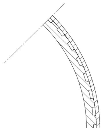
**Cross-section of the shower DWHR unit with leak detection ducts.**
